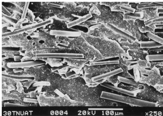
Figure 10 SEM photomicrograph of unaged composite. Debonding and fiber pullout are visible.
